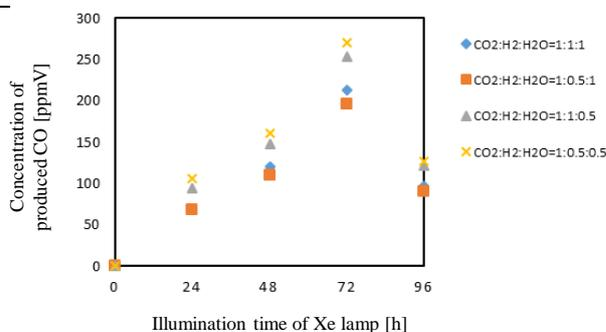
Figure 1. Comparison of CO<sub>2</sub> reduction performance of Cu/TiO<sub>2</sub> film under illumination conditions without UV light.
