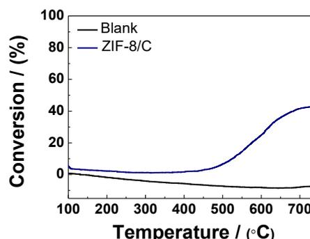
**Figure 1.** CO<sub>2</sub> conversion with temperature for ZIF-8/C.
