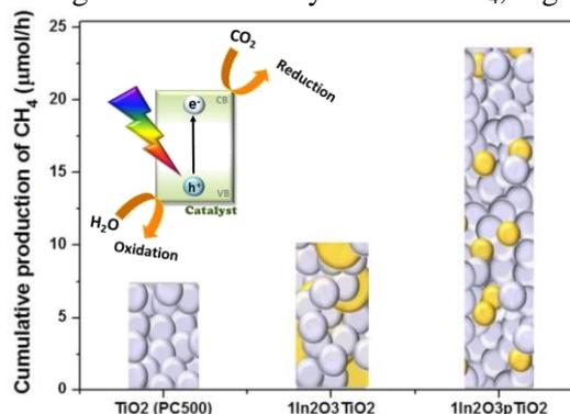
Figure 1. Cumulative production of CH<sub>4</sub> for TiO<sub>2</sub>, 1In<sub>2</sub>O<sub>3</sub>/TiO<sub>2</sub> and 1In<sub>2</sub>O<sub>3</sub>p/TiO<sub>2</sub> catalysts.
