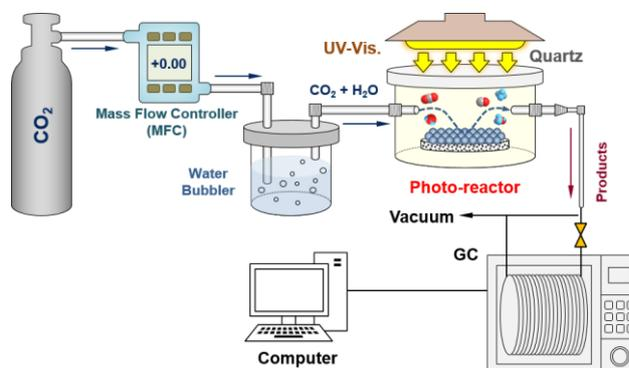
Figure 1. Experimental setup for photocatalytic conversion of CO<sub>2</sub>
