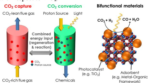
**Figure 1.** Schematic of a combined CO<sub>2</sub> capture and photocatalytic conversion process using bifunctional materials
