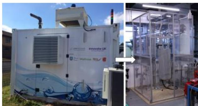
**Figure 1.** Pilot plant for the novel low-carbon Haber-Bosch synthesis of ammonia.
