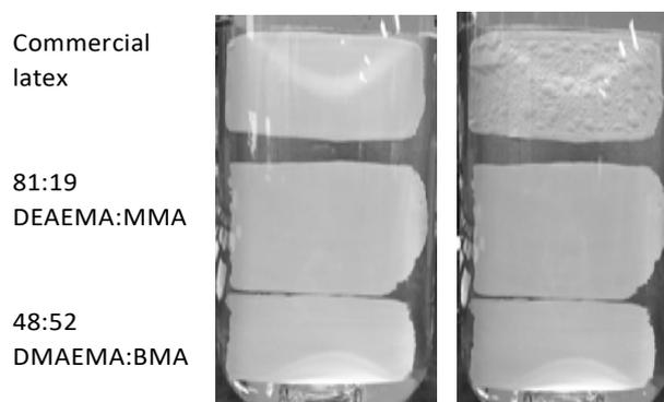
**Figure 2.** The stability of dried CO<sub>2</sub>-responsive materials and commercially water-based latex after immersion in water for one week.
