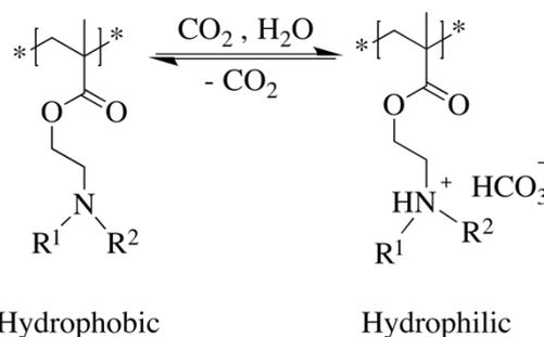
**Figure 1.** CO<sub>2</sub>-responsive polymeric amines are hydrophobic in the absence of CO<sub>2</sub> and water but are hydrophilic in the presence of CO<sub>2</sub> and water.
