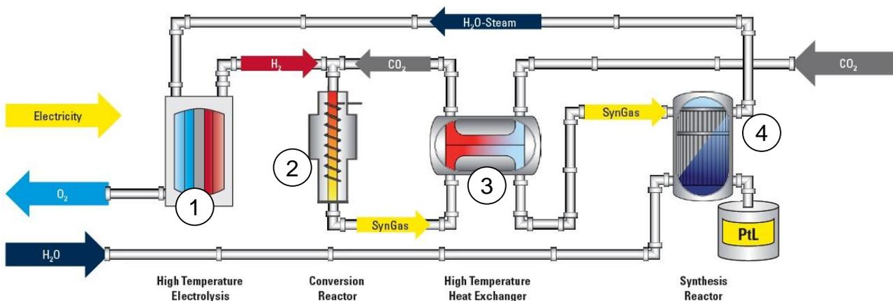
Figure 1. Sunfire Power-to-Liquid process [2].
